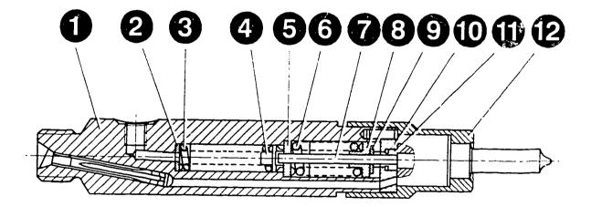
As soon as the prestroke H1 has been completed and the needle valve has caused the stop sleeve (11) to make contact with the intermediate disc (10), a second pressure spring (6) comes into effect.
